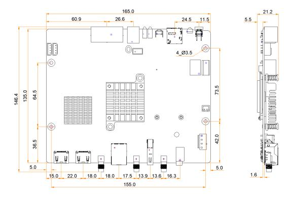
Tolerance: ±0.3 Unit: mm
